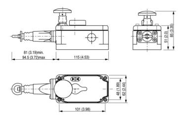
Extended Length Models (75...125 m cable span)
