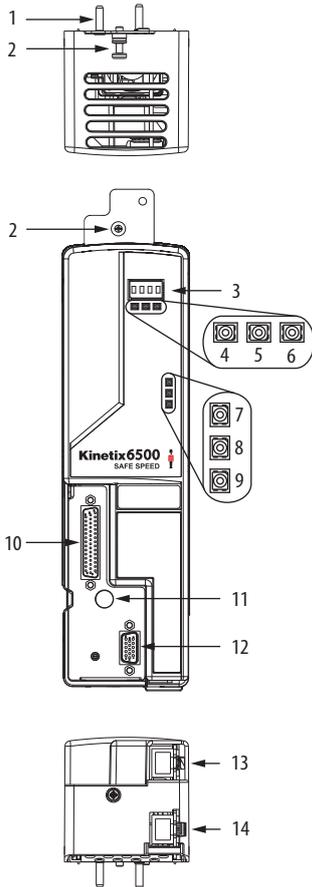
**Control Module (2094-EN02D-M01-5x) Top View**
